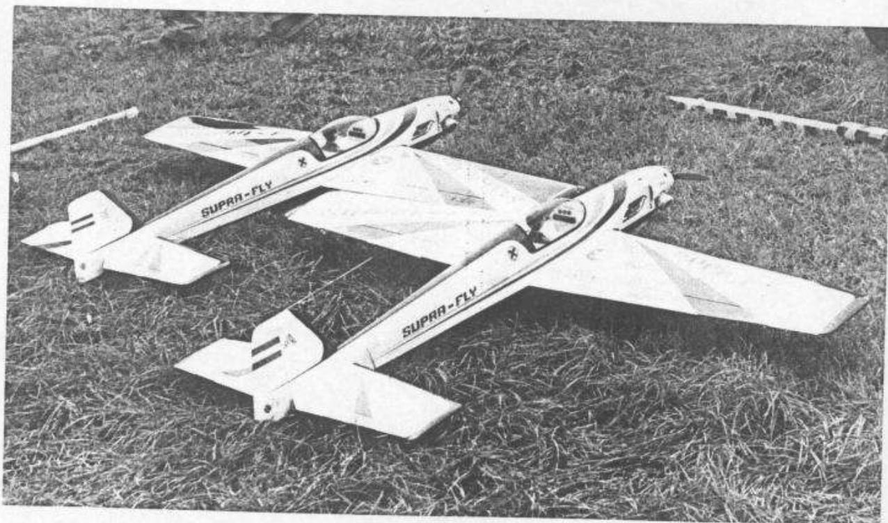
Here, again, are Hanno Prettnner's Supra Fly's (A and B ships). Their design is quite similar to the earlier Calypso but with larger tail surfaces.
