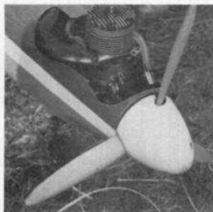
Below: the Swiss Landert variable pitch prop, as used by Wolfgang Matt in the fly-off is fully variable from -5^{\circ} to +10^{\circ} . The blades appear to be glass filled nylon, while the mechanism is built into the nylon spinner. Diagram of the unit from the manufacturer's instruction sheet, is seen at bottom of this page. The unit is available in U.K. through Slough Radio. Control price, £63.95.
