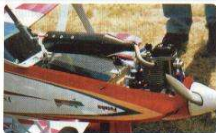
Prototype Asano exhaust in the Narlar biplane. Note check valve fitted to DZ injector to help throttling from low engine speeds
