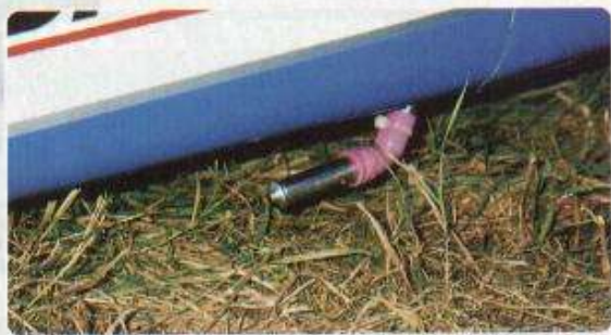
Exhaust diffuser on the 'Good Shot' used to reduce exhaust orifice noise levels to good effect
