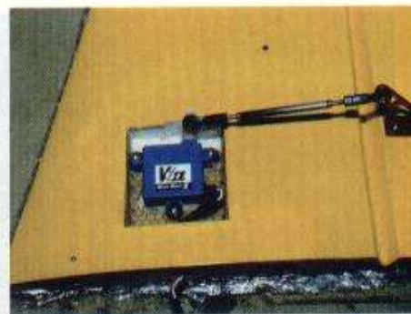
Martin used the Volz 'Micro-Max X' servos for elevator control. He found the elevator very responsive at first.
