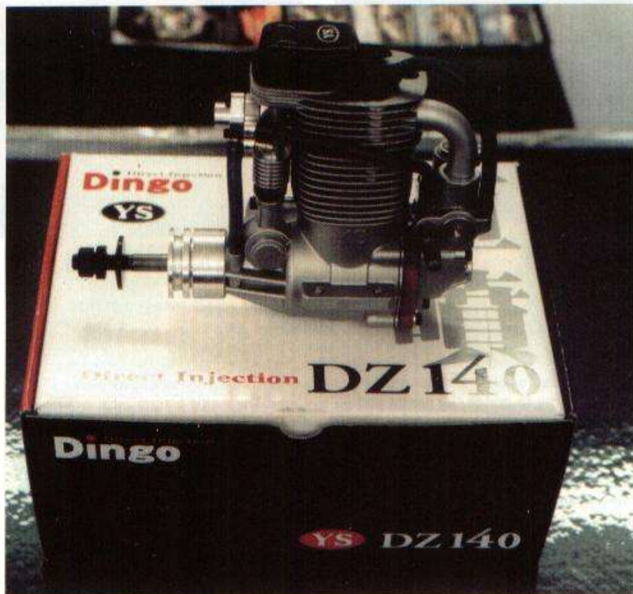
Front view of the new 1.40 engine, the regulator and mechanical pump is now located on the inlet valve push rod cover and driven by the inlet push rod.
