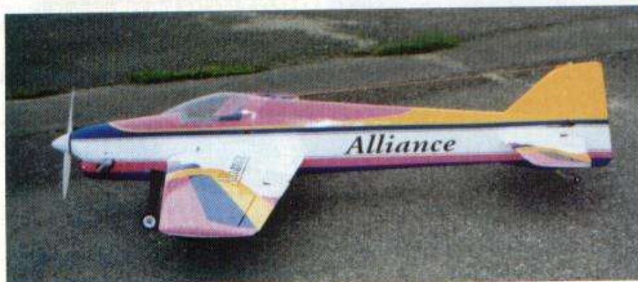
Mk Alliance designed around the popular YS.63 engine. As can be seen the model is simple in its layout, with the silencer just exiting out the side of the cowl.
