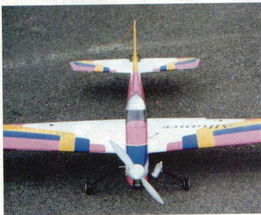
Front view of the Alliance showing the wide track of the fixed gear.
