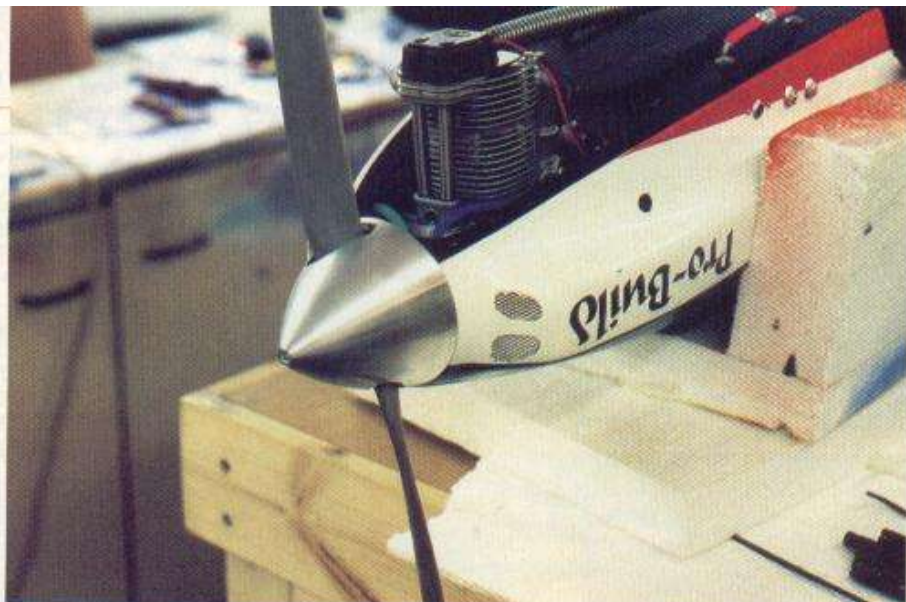
The YS 140LM installed in the front of the model, many people have asked what the material is I use in the air inlets. The material is aluminium used to patch holes in cars with filler; it can be obtained from any car parts shop and costs about £1.00.
