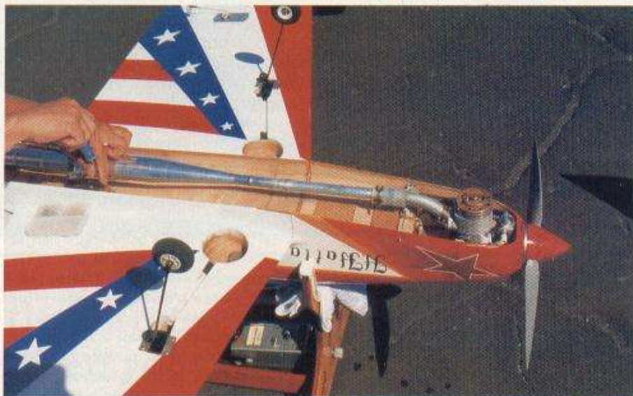
Hatta's model again this time with the underbelly removed to show the installation of the OS 140 with a twin plug head fitted. Note also the models are built out of balsa and then spray finished.
